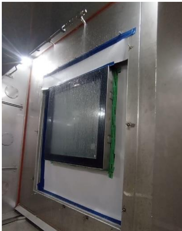
Fig. 5 Water tightness test in progress
